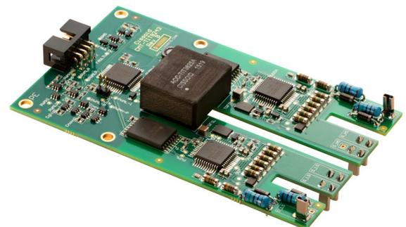
Figure 2: CMT-TIT8243 high temperature high voltage isolated Gate Driver
